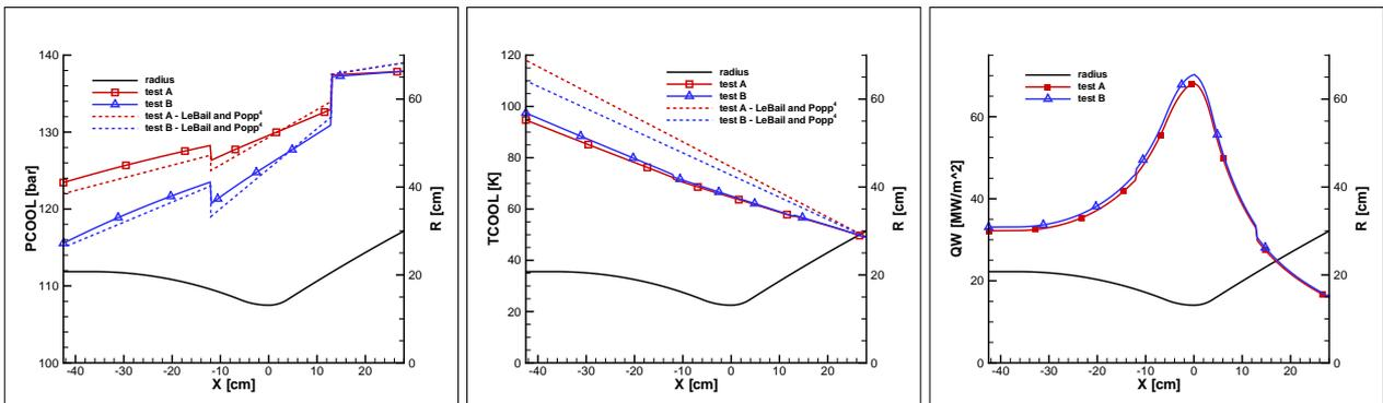
Figure 3: Coolant pressure (left), coolant temperature (center) and wall heat flux (right) for tests A and B.
