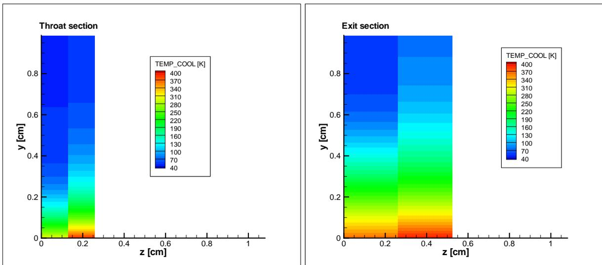
Figure 5: Coolant and fin temperature stratification at throat (left) and exit (right) section for test case A.
