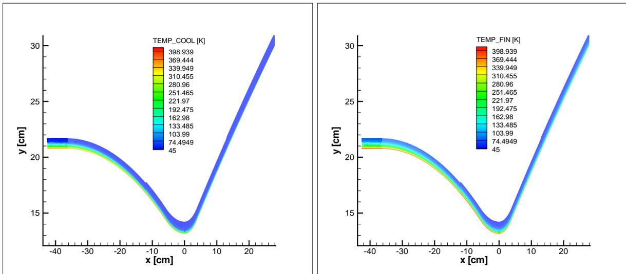
Figure 4: Coolant (left) and fin (right) temperature stratification for test case A.
