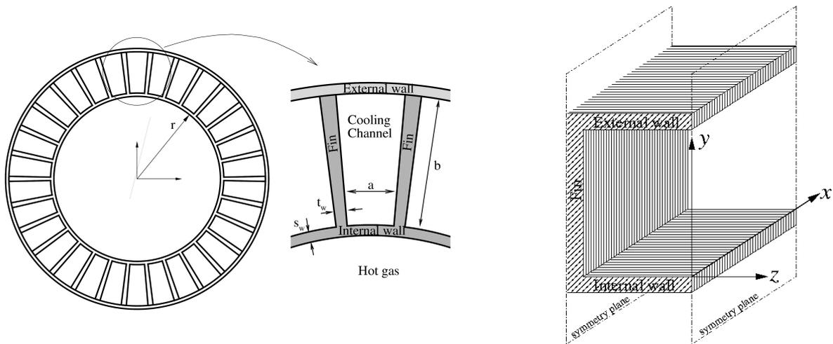
Figure 1: Schematic of cooling channels geometry.
