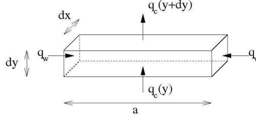
Figure 2: Heat fluxes in a slice of cooling channel of width  $a$  and height  $dy$ .
