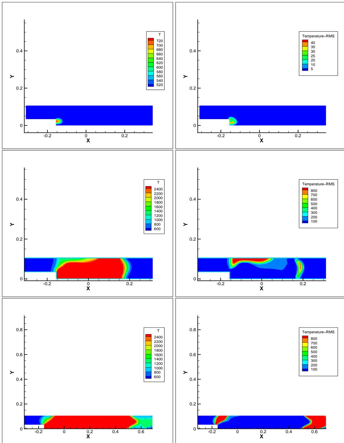
Figure 2: Instantaneous snapshots of the mean temperature (left column) and root mean square temperature (right column) for 10, 2000 and 6000 iterations (from top to bottom)
