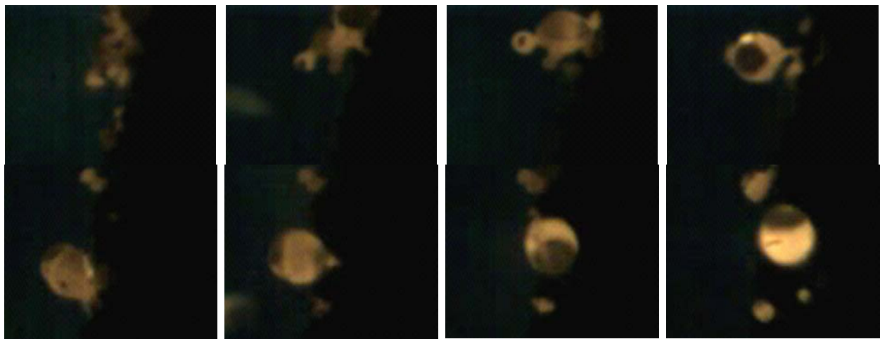
Figure 6: Aggregate/agglomerate mechanism evolution on the burning surface of 5% \text{AlH}_3 sample
