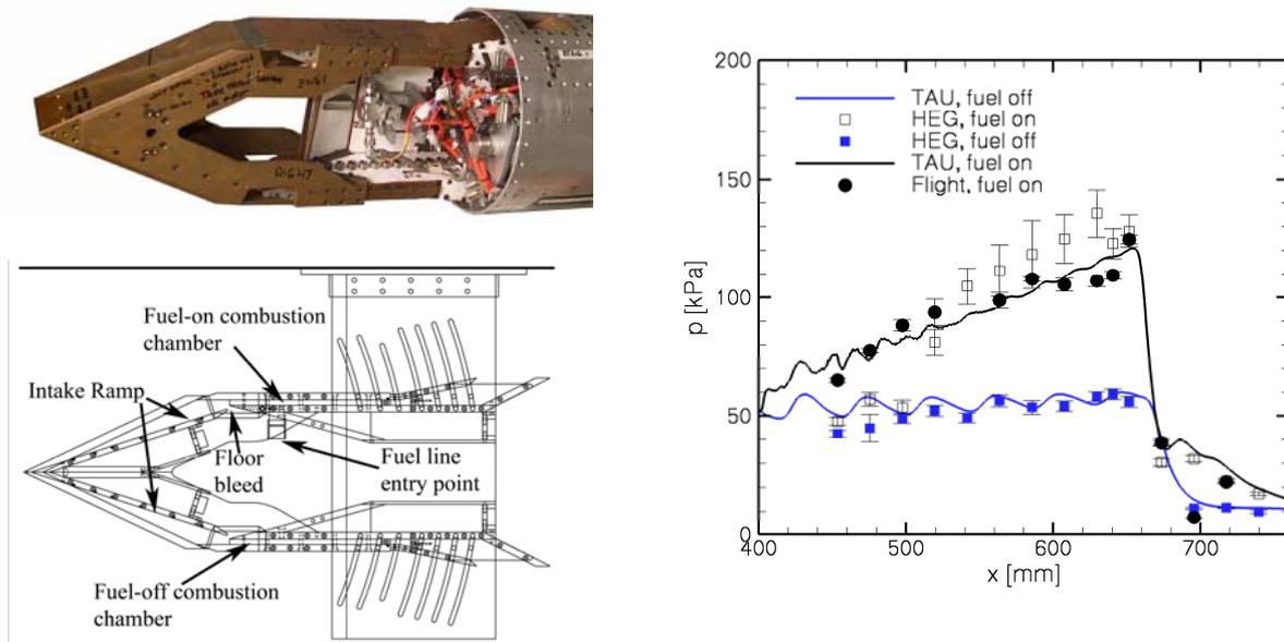
Figure 9: Photograph of the HyShot flight configuration (courtesy The University of Queensland, Australia) and schematic of the wind tunnel model (left); Measured and computed static wall pressure distributions in the HyShot combustor at a flight altitude of 33 km (right).
