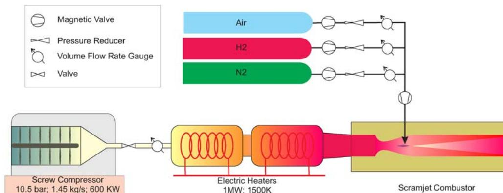
Figure 1: Schematic of the supersonic combustion test facility of ITLR at Universität Stuttgart.
