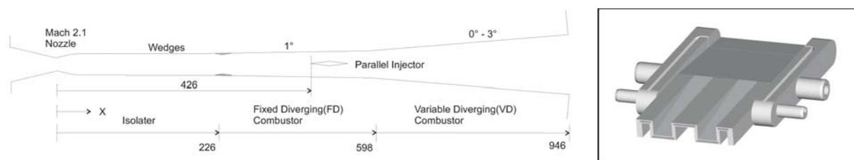
Figure 2: Schematic of the test section and combustor configuration (left) and of the lobed injector (right) used in [6].
