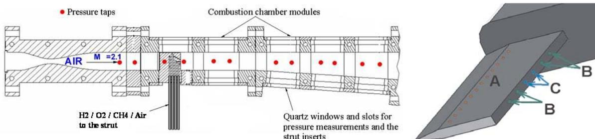
Figure 4: Side view of the modular combustion chamber with strut injection (left) and strut injector (right) [15].
