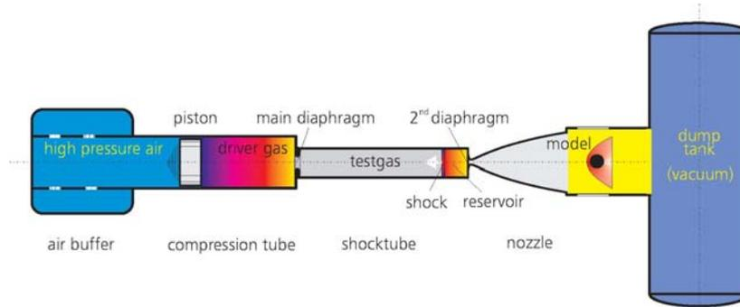
Figure 8: Schematic of the free piston driven shock tunnel, HEG (not to scale).
