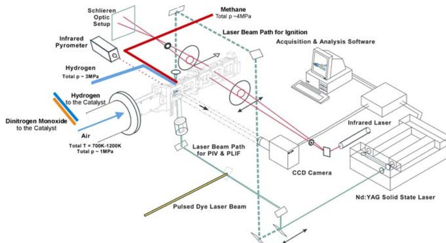
Figure 3: Schematic of the connected tube test facility of the Institute of Flight Propulsion [see e.g. 10].
