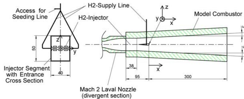
Figure 6: Combustion chamber dimensions and injector installation in the M11-4 facility [19].
