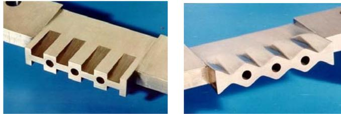
Figure 7: Fuel injectors USCER (left) and WAVE (right) used in the M11-4 facility [19, 20].
