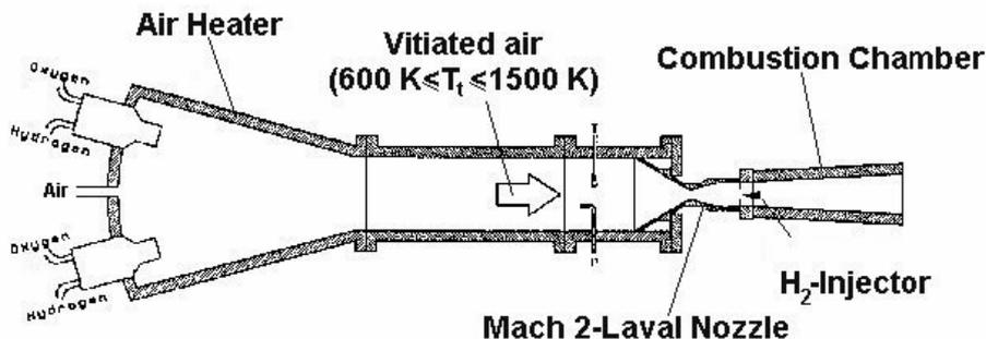
Figure 5: Schematic of the connected tube facility M11-4 at DLR Lampoldshausen (not to scale) [19].
