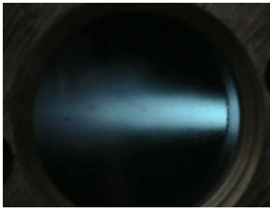
Figure 15: Flame jet issuing from the igniter nozzle at ignition energy of 100 mJ
