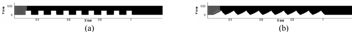
Figure 1: Shock wave enters the channel section with regular orifice plates (a) and with regular shaped obstacles (b). Only a lower part of the channel is shown in the figure
