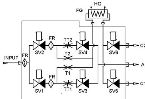
Figure 2: GDU functional schematics
