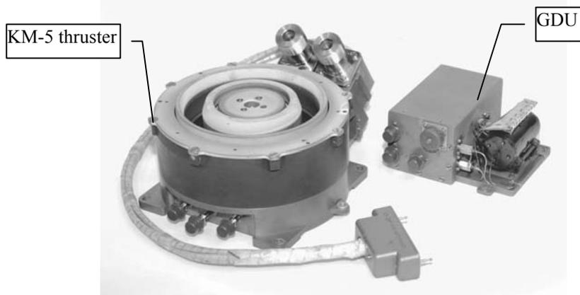
Figure 1: Hall thruster KM-5 and gas distribution unit
