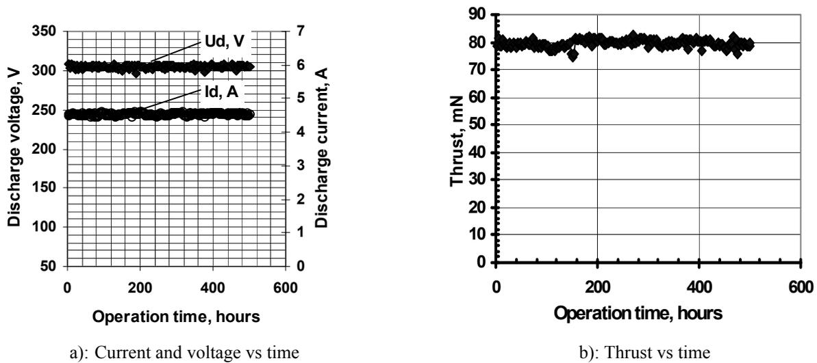
Figure 3: Evolution of parameters during the life test
