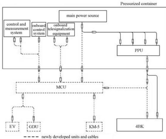
Figure 5: Block diagram of the electrical interface and APU circuit connection
