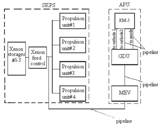
Figure 6: Diagram of APU and SKPS pneumatic circuit connection
