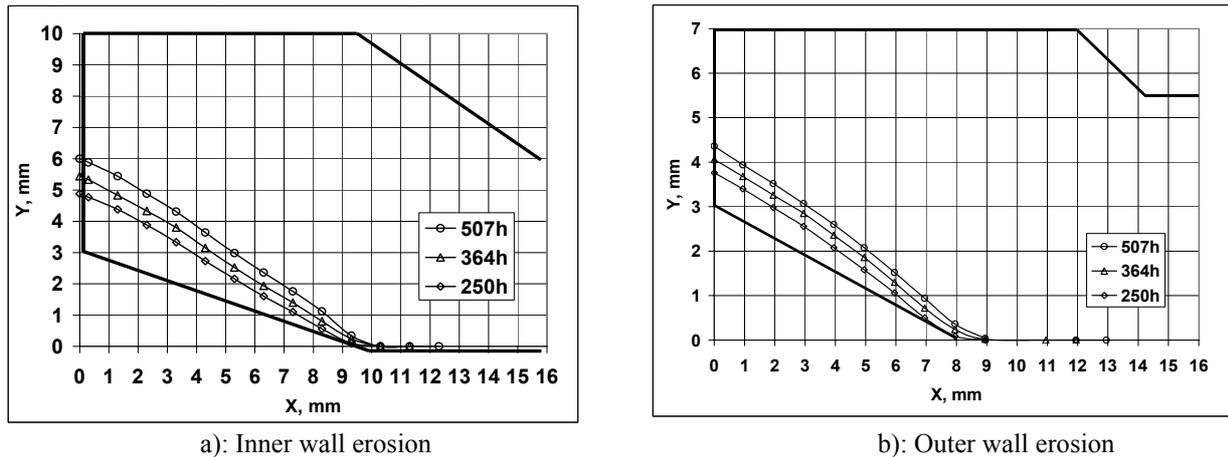
Figure 4: Insulator profile change during the life test
