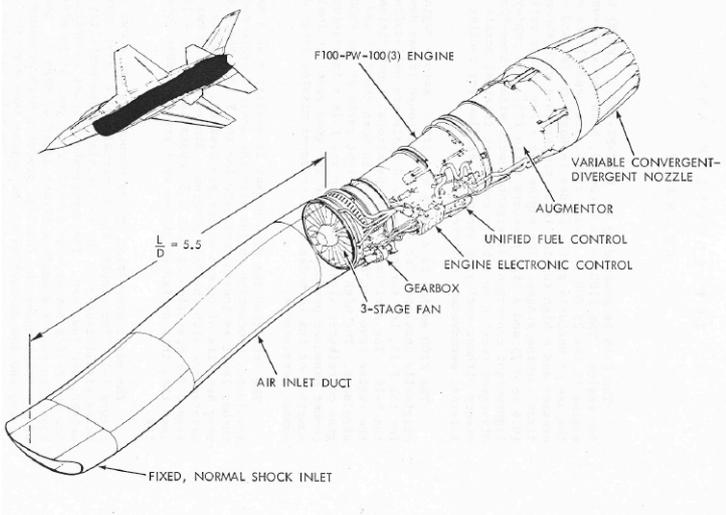
Figure 2 – The F100 in the F16 with its belly-mounted intake
