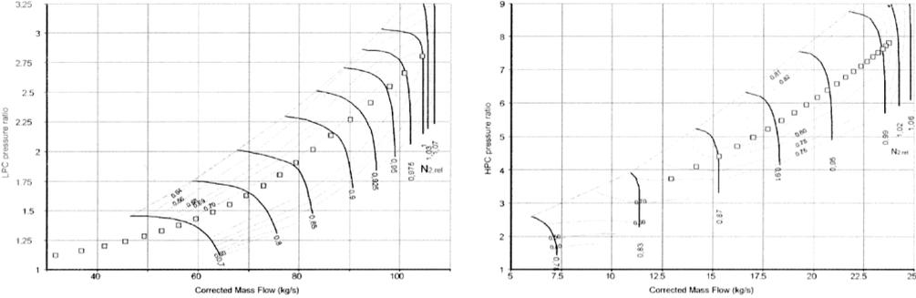
Figure 1 – Steady state line on the LPC (fan) and HPC maps
