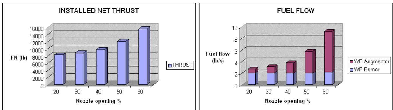
Figure 5 – Afterburning influence on the installed net thrust and the fuel flows (Ma = 0,82, 20.000 ft ISA)
