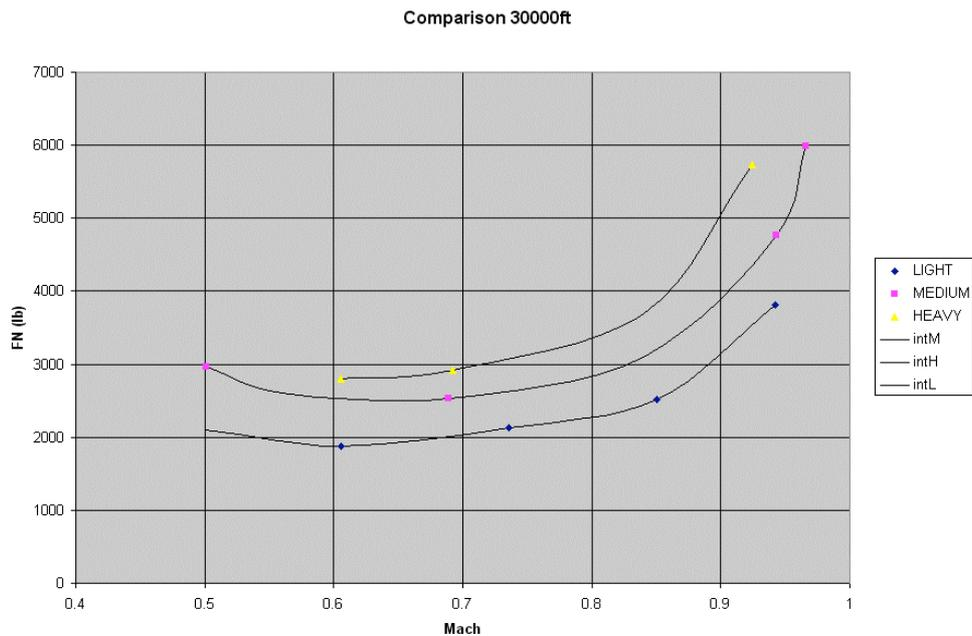
Figure 6 – Requested thrust evolution for three different aircraft configurations
