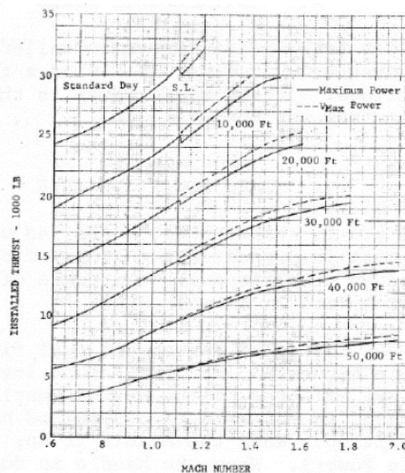
Figure 4 – Available installed performance of the engine
