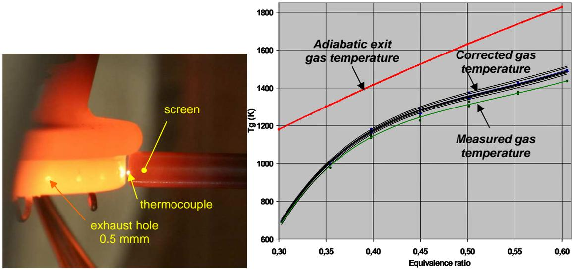
Figure 4: Exit gas temperature measured by thermocouple (0.25 mm diameter) - Mass flow rate 0.4 g/s.
