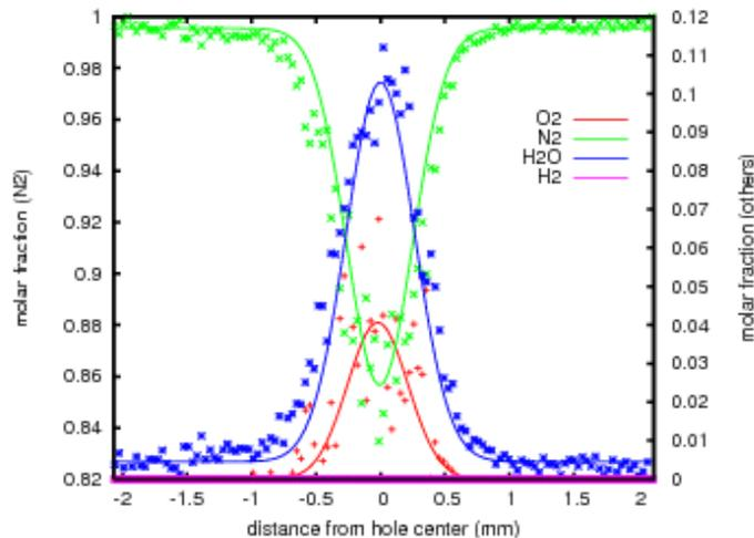
Figure 7: Radial profiles of molar fractions in the burnt gases jet (air mass flow rate: 0.1 g/s,  $\Phi=0.4$ ).
