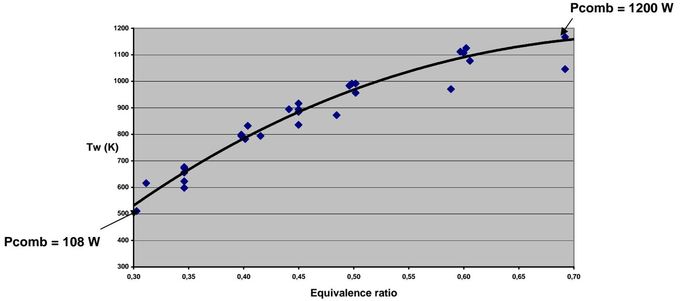
Figure 3: Mean wall temperature for the range of operating conditions.
