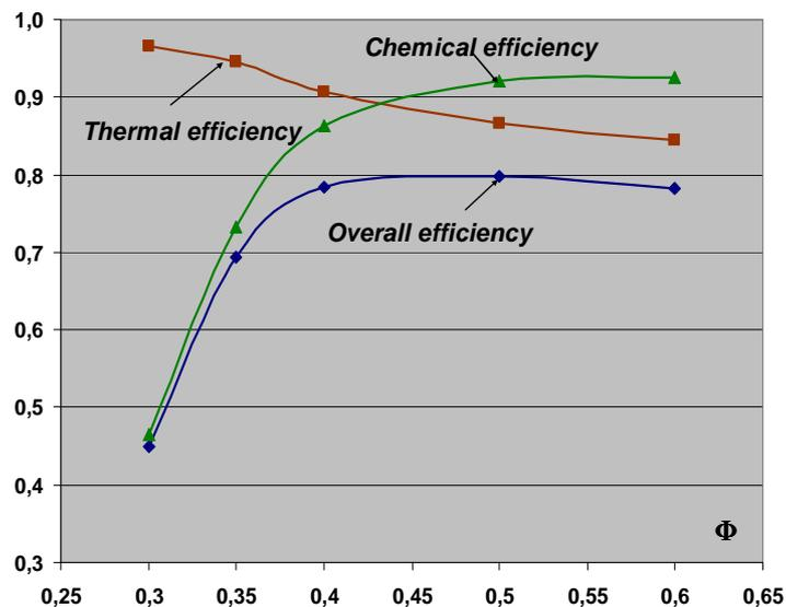
Figure 5: Overall, thermal and chemical efficiencies versus equivalence ratio - Air mass flow rate: 0.4 g/s.
