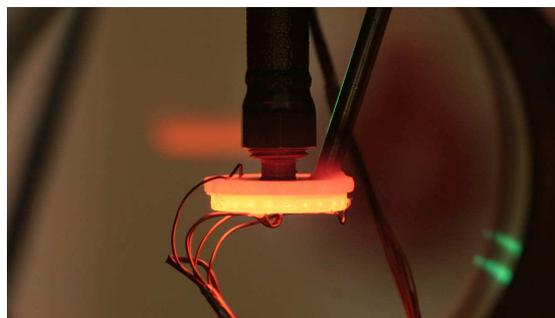
Figure 2: Firing micro combustor.
