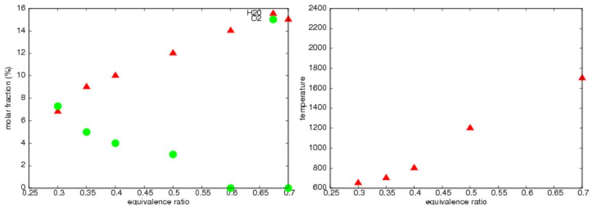
Figure 8: Molar fractions and temperature vs. E.R. for 0.1 g/s air mass flow rate.
