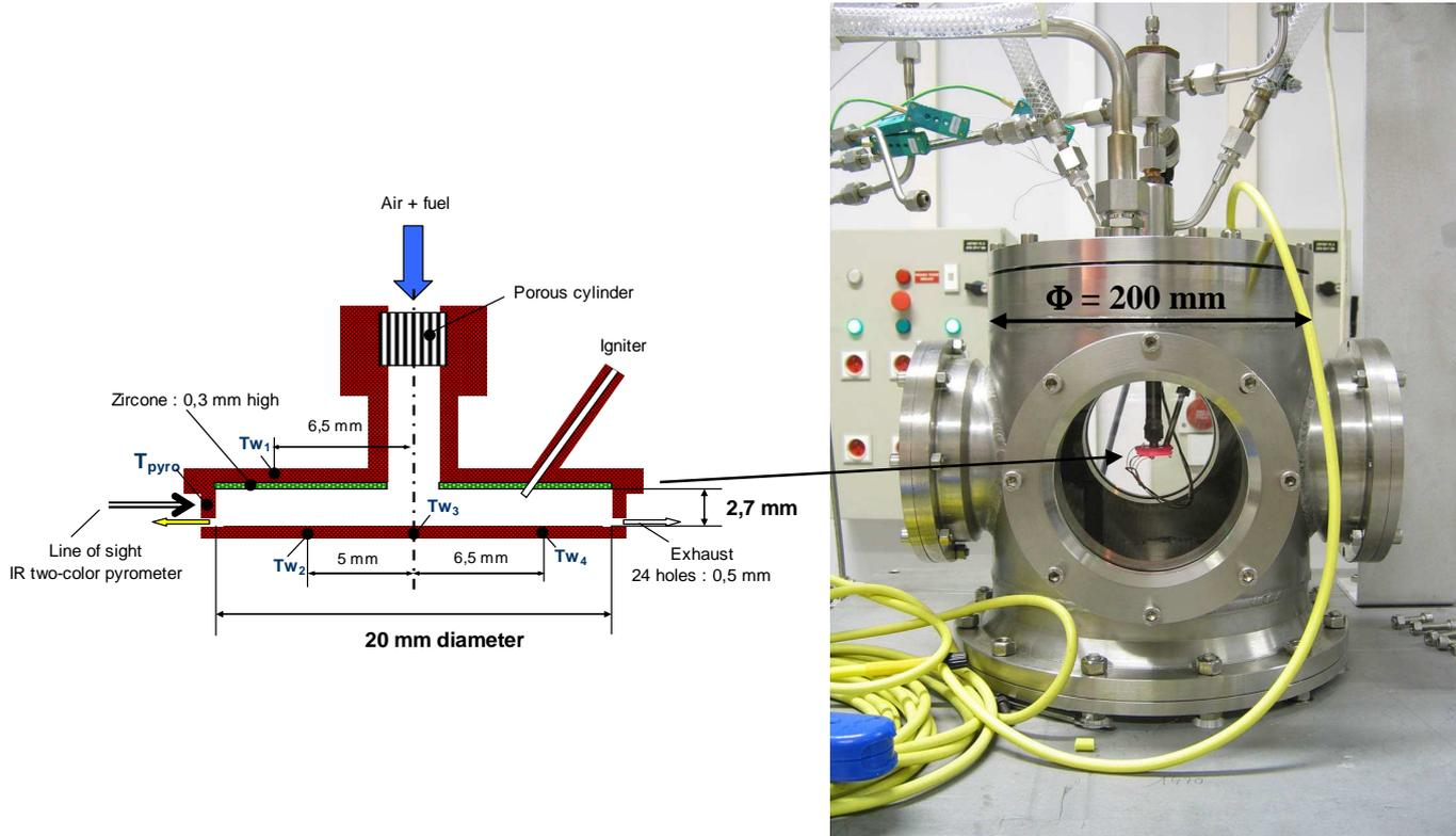
Figure 1: Cross-section of the first micro combustor and its position in the pressurized vessel.
