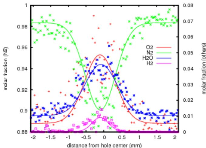
Figure 9: Radial profiles of molar fractions in the burnt gases jet (air mass flow rate: 0.4 g/s,  $\Phi=0.35$ ).
