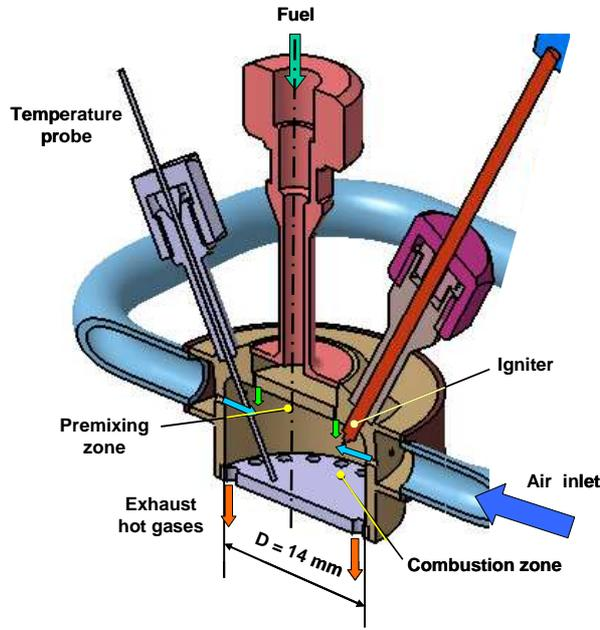
Figure 10: Second micro-combustor – Non-premixed case.
