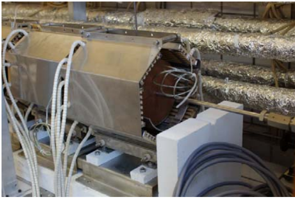
Fig. 3 – Basic experiment on endothermic fuel reforming at ONERA
