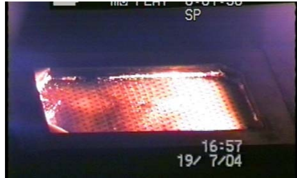
Fig.1 – Example of fuel-cooled panel tested in 2004
