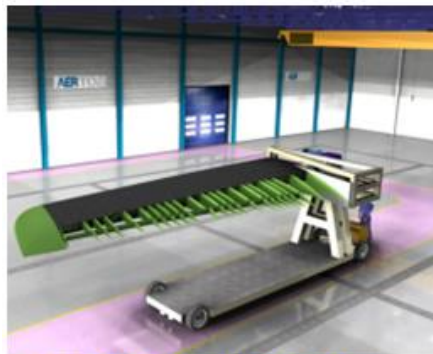
Smart Wing semi-assembly ground transportation (Aernnova)
