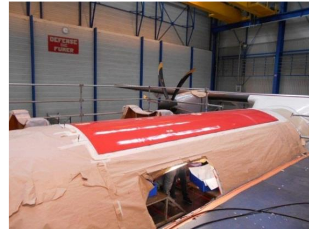
CFRP Stiffened Panel mounted on Crown Fuselage
