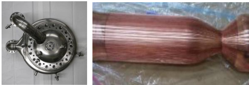
Figure 10. Injector and Combustion Chamber Inner Part
